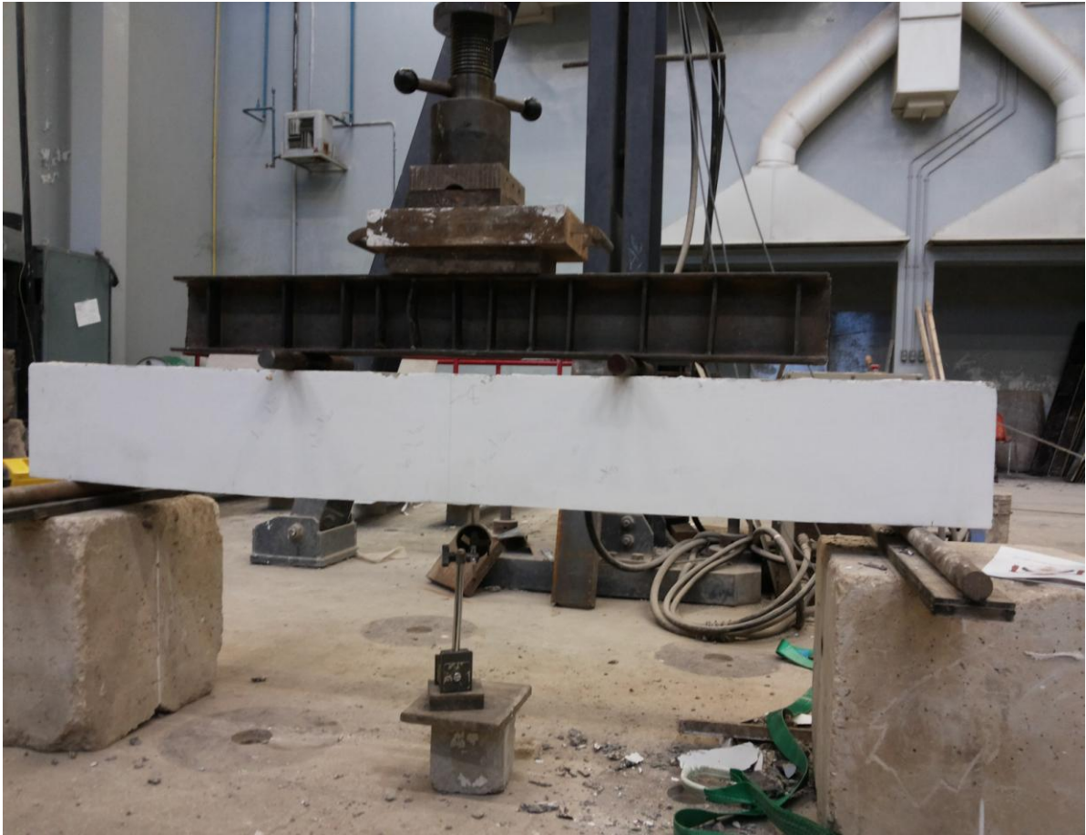
Figure 4: Experimental set up and crack monitoring
